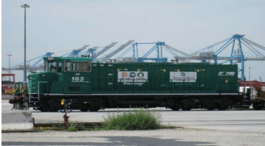
One of two multi gen-set locomotives at NIT
